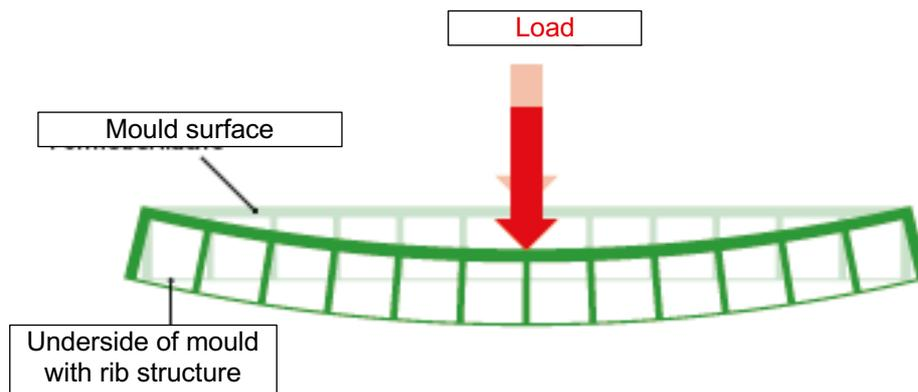
Figure 4. Schematic illustration of the loading case critical for crack formation
