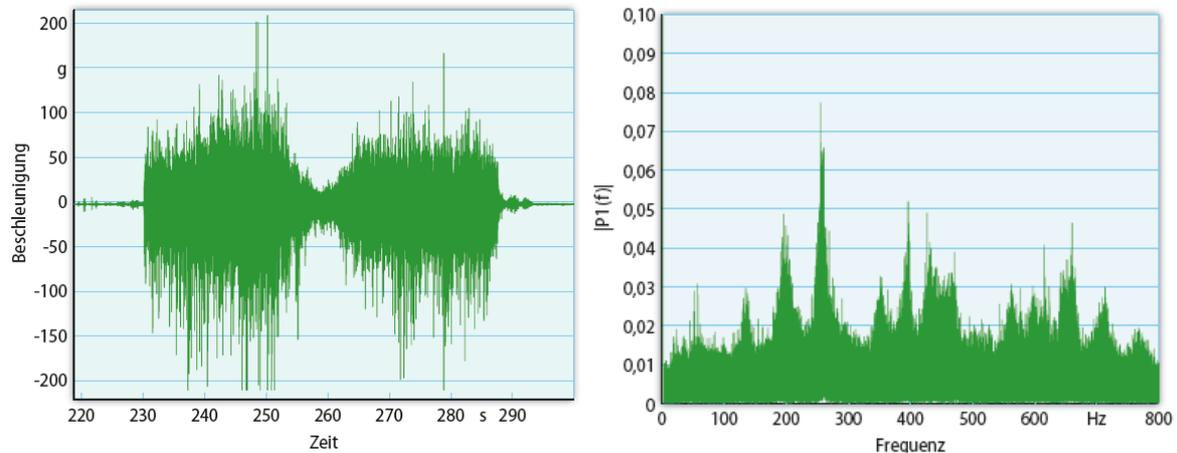
Figure 1. Recorded acceleration values in the vertical direction (left) and illustration of the frequency spectrum (right)
