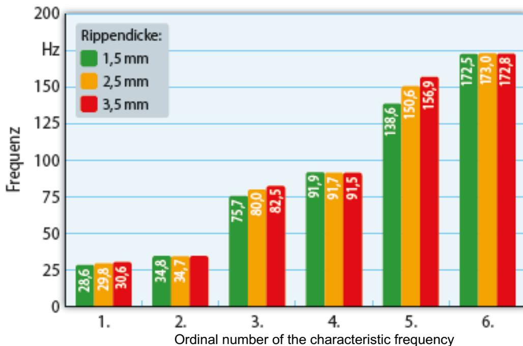
Figure 2. Illustration of the first six characteristic frequencies of a chocolate mould with various different rib thicknesses
