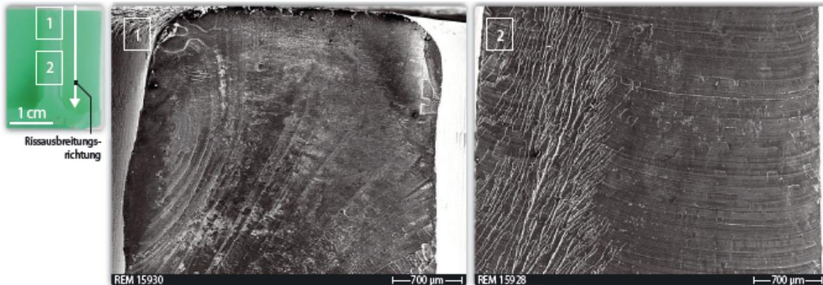
Figure 3. Fully opened-up crack (left) with crack propagation direction and SEM images of the marked positions. The crack initiation (1) and cyclical crack propagation can be identified on the basis of the arrest lines (2) Source: Crack propagation direction
